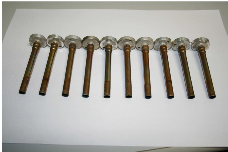
Fig.3 Igniters are not deformed and no signs of fly-off effect after shooting
