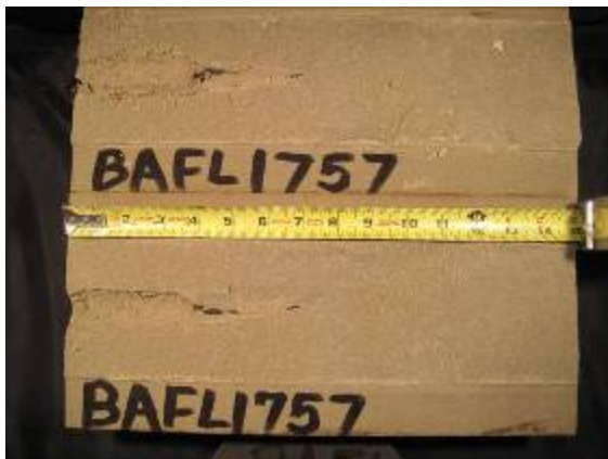
23g HMX GH in sandstone
