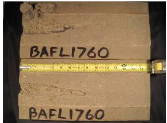
23g HMX GH DPEX in sandstone
